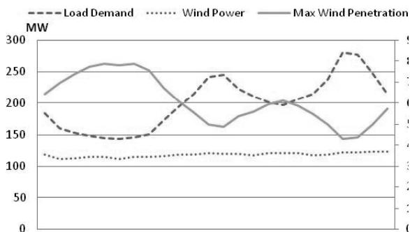
Fig. 10. Max recorded penetration in a 24-hours profile
