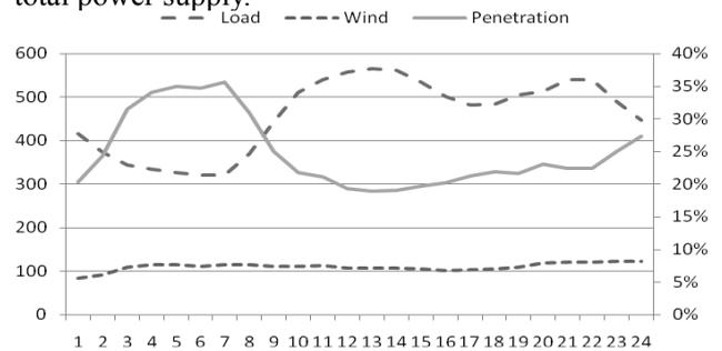
Fig. 7. Wind power penetration in power system of Crete
