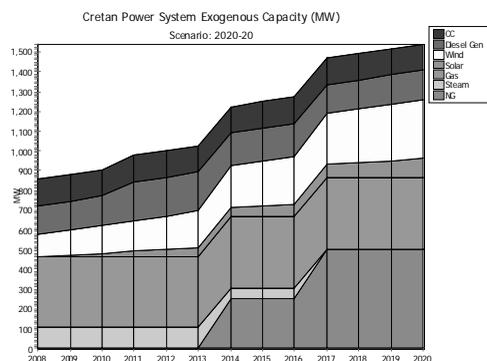
Fig. 13. Installed capacity evolution
